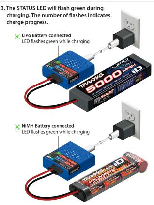
Note: It is normal for the charger to become warm while charging at the maximum charge rate. If the charger is not in a cool, well-ventilated area, the charge rate will be automatically reduced to prevent the charger from overheating.
